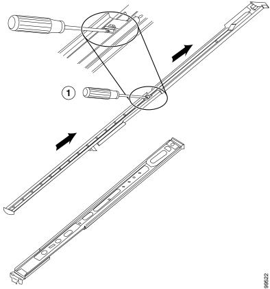
4. Select a location in the rack to mount the GSS and attach the front end of the right outer telescopic rail to the right side of the rack, as show in Figure 3-4.
